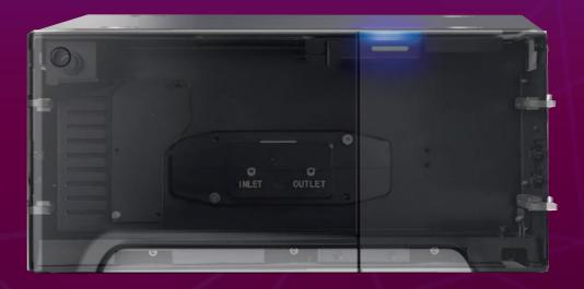
Ultra-high sensitivity, low dispersion total reflection flow cell Optical path length matches ultra-high performance analysis requirements
